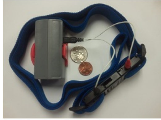
Figure 2: Respiratory Inductive Plethysmograph band (in blue color) is worn around the chest area and the wearable AutoSense sensor unit clips to the belt. A 3-axis Accelerometer, ECG, and Galvanic Skin Response sensors are also included in the same sensor unit. Two coins (a quarter and a penny) are also shown in the picture to indicate the form factor.
